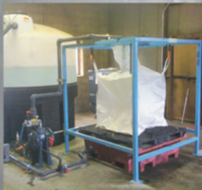
This is a Bag Filter module that is installed at a stone shop in Ontario. The bag system can be used in conjunction with the filter press, and act as a primary sedimentation module. The bag system will gather the heavier solids which will allow the filter press to perform longer without maintenance.
