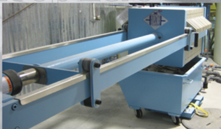
The Hy-Pack filter press is manufactured in our 45,000 square foot facility in Kenosha, Wisconsin, and sized appropriately for your specific needs. All of our filter presses are expandable to grow with your business. The Hy-Pack filter presses are steel frame construction with polypropylene filter plates, and filter cloths designed for your needs.
