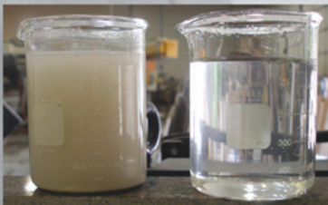
These are actual water samples before and after processing with a Beckart Environmental filtration system at a stone fabricating facility. Our systems will filter the water down between 1 and 2 microns at water flows of up to 200 GPM.
