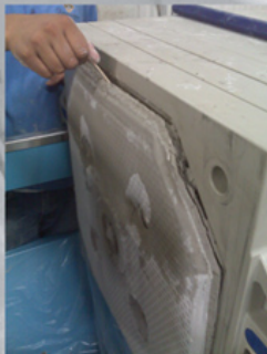
Above is a sample of a typical dry and compacted filter cake after water filtration with a Beckart Environmental filtration system.
