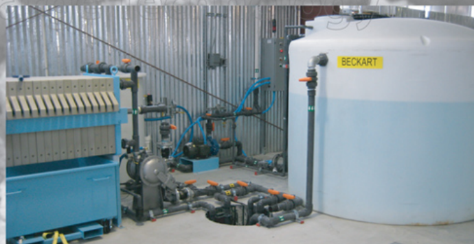
Beckart's optional PLC automation with graphic operator interface allows the user to input the flow rate needed and the PLC (programmable logic controller) will automatically step up the air pressure as the filter press fills up to constantly give you the clean water your machines require without the hassle of manually increasing the air supply. All Beckart electrical control panels are assembled and programmed in-house to insure the highest level of quality.
