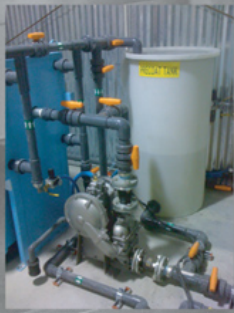
This is a Sludge / Precoat pump system with precoat tank and Beckart Hy-Pack filter press in a fabrication shop in Virginia. We have fine tuned the precoat process to insure thorough coating.
